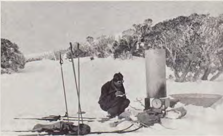
Reading a snow gauge near Mt. Cope. Note the scales mounted on a toboggan.
